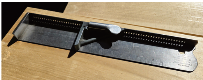
Using a composing stick like the one shown here you set the length of the lines that you want, then insert your type upside down and backwards.
