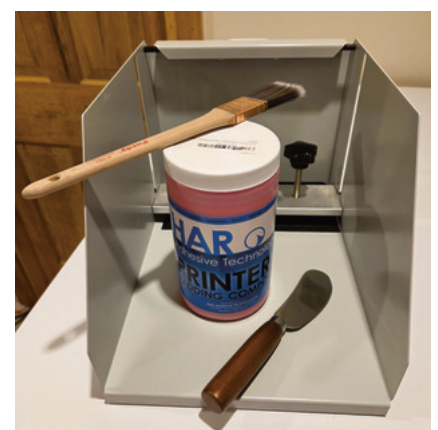
Brian's padding press along with padding compound, a brush, and a knife for separating the completed pads. This is the side from which you load the printed sheets. The panel toward the back is removed. The padding compound is painted onto that edge of the paper
